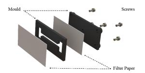
Figure 1: Exploded view of Alginate Mould
