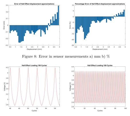
Figure 9: Loading cycles of Hall effect sensor a) 5 b) 100
