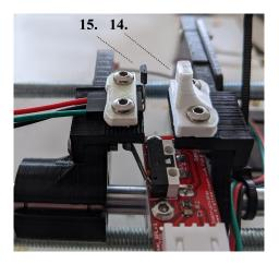
Figure 4: Hall Effect Sensor and Magnet Mounting
