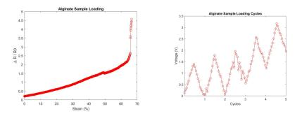
Figure 5: a) Loading of Alginate sample b) 5 Alginate Sample loading cycles at 10% strain
